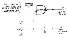
fig. 4. Simple rf amplifier using a TTL NAND gate. Rf output is about 2 volts p-p for 100 mV p-p input.
